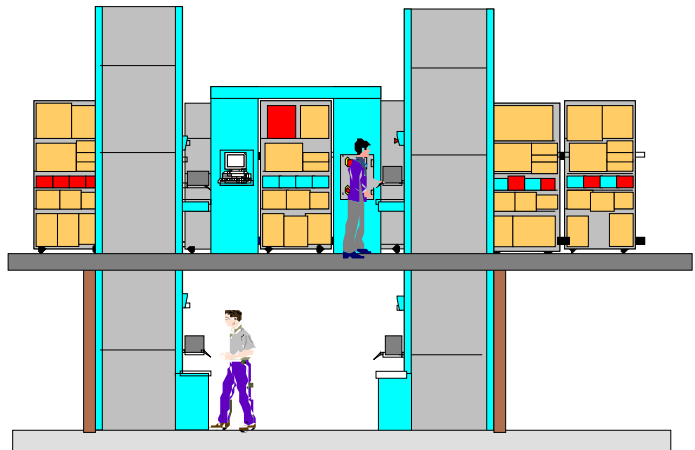
Installation with a Horizontal Carousel on a mezzanine floor with two Vertical Carousels installed through the floor.
