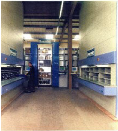
Installation with a Horizontal Carousel on a mezzanine floor with two Vertical Carousels installed through the floor.
