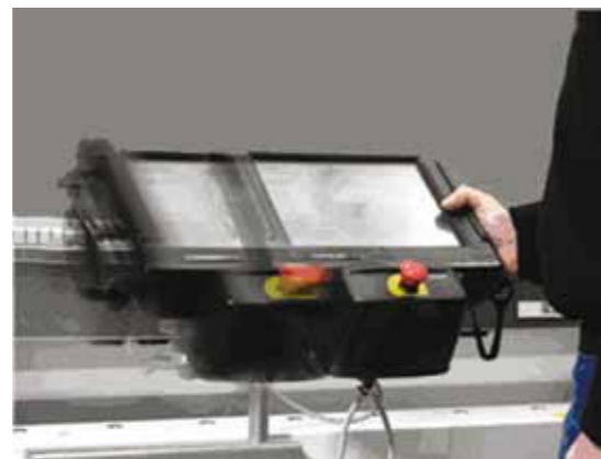
Sliding console moves along the tray length
