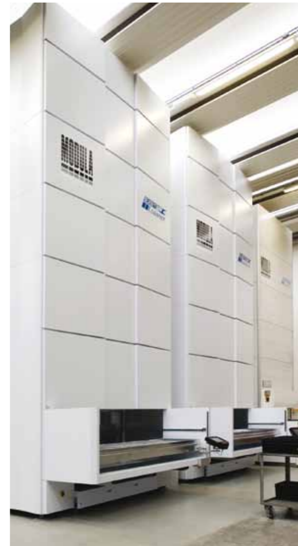
Internal tray presentation includes autodoors as standard
