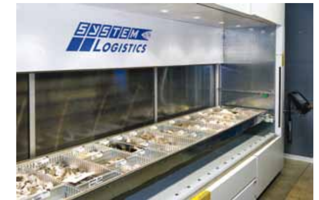
Internal tray presentation includes autodoors as standard
