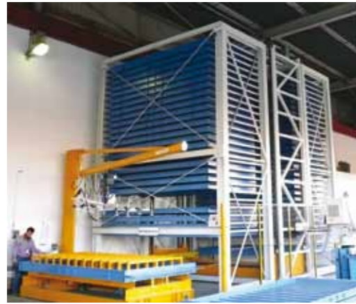
Cassette for 4m x 2m sheet steel
